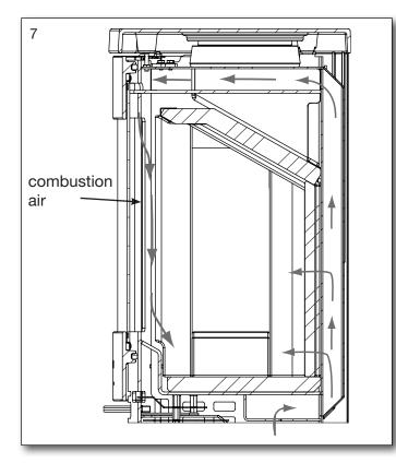
Minimum chimney draft: 11 PA. It is the draft that the stove has been tested and approved on. The minimum draft is necessary to provide clean burning, beautiful flame picture, as well as achieving the rated efficiency.
