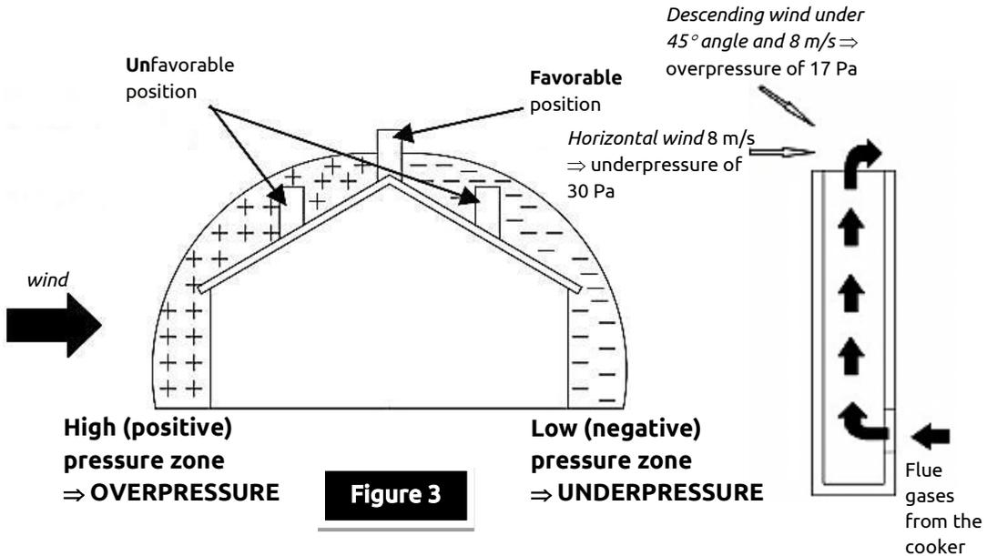
The wind also influences the chimney function indirectly by creating areas of high (overpressure) and low (underpressure) pressure, both inside and outside the residential area (Figure 4).
