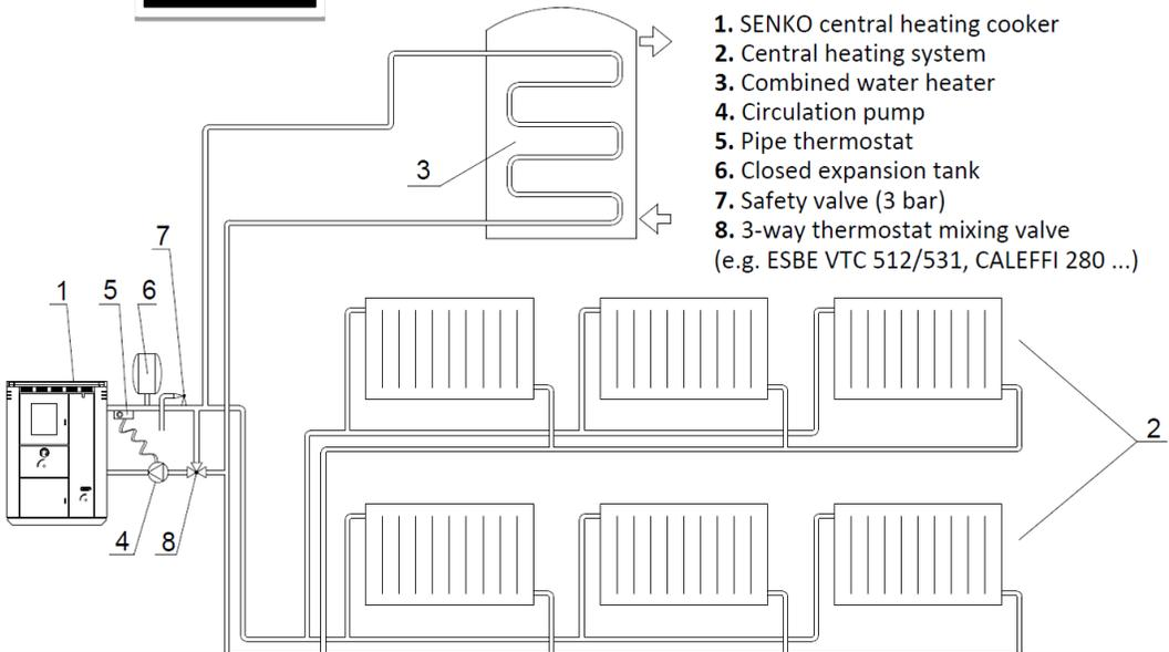
It is necessary to **install the deaerating valve**. When filling the boiler and the radiator system it is necessary to open the mixing valve, if one had been installed; adequately deaerate the boiler and the heating system.
