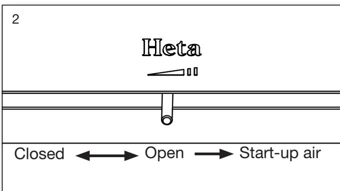
The Scan-Line Solid C stoves are designed and tested to burn extremely cleanly with very little smoke discharge and are exempt for use in smoke control areas throughout the UK when burning dry wood logs. To comply, a permanent stop is fitted to ensure that the air control slider cannot be closed beyond (percentage of air as per test) of its fully open position. A permanent
