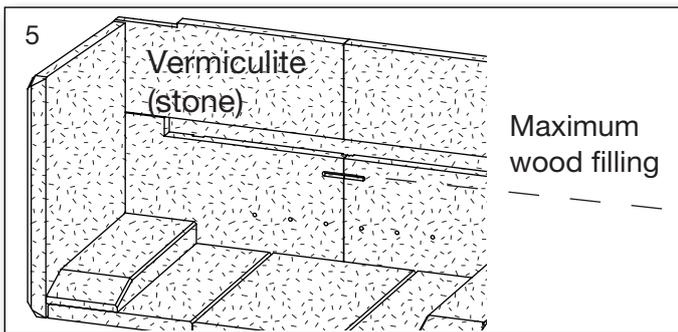
The fuel load, must be maintained below the top series of air holes and within the outer vent in each side. Fig. 5
