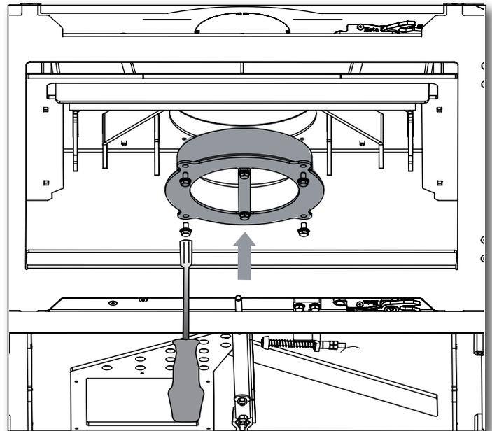
The flue collar is bolted to the stove from inside the fire chamber with, 4 x M6x10 0008-1117.
