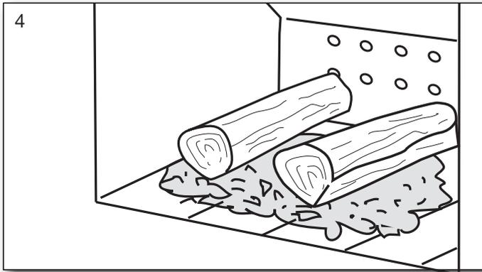
The wood will then ignite within a very short time (Typically 1 to 3 minutes). Once the fuel is ignited. Close the door and regulate the air back to operating air. When the fire is well established, you can now regulate the operating air to the desired combustion level.
