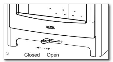
fitted to ensure that the air control slider cannot be closed beyond 33% for Ambition 5 and 42% for Ambition 8 of its fully open position. A permanent amount of air will therefore enter the firebox to feed the fire producing negligible amounts of smoke and unburnt hydrocarbons. The appliances will only be considered as an exempt appliance if this stop is in place.
