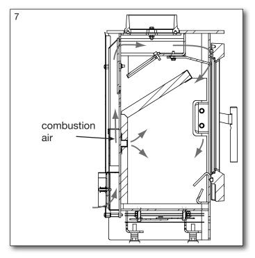
that it itself provides an optimal blend of combustion air. This provides a high efficiency/heat, clean glass and low environmental impact.
