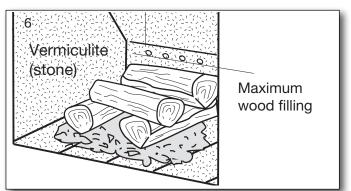
The fuel load, must be maintained below the top series of air holes and within the outer vent in each side. Fig. 6.
