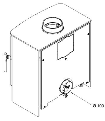
When installing external air supply, connect the air intake to the direct air pipe using flexi-pipe,
