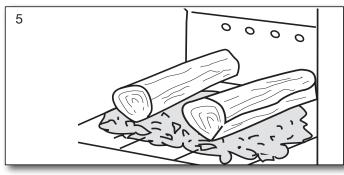
front. Place pieces of wood equivalent to about 1,2 kg for Ambition 5 and 1.8 kg for Ambition 8 on top of the embers perpendicular to the door. See fig. 5.
