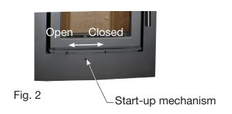
up airflow for the stove, push the handle on the start-up mechanism as far to the right-hand side of the stove (as seen from the front) as possible.
