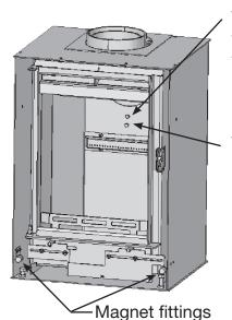
The top screw has to go through both the combustions chamber and the convection box.
